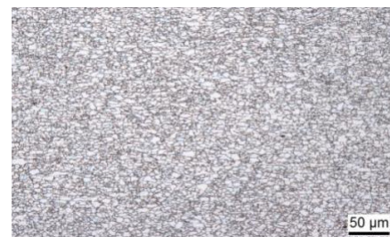
Figure 1: Microstructure images S420GD, resolution 200:1
