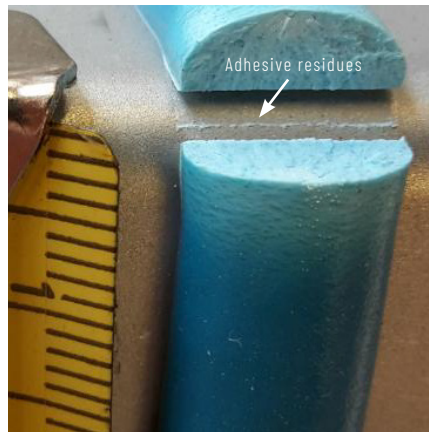
Figure 4: Zinc adhesion test for a S420GD+Z275, adhesive bead test according to VDA test sheet
